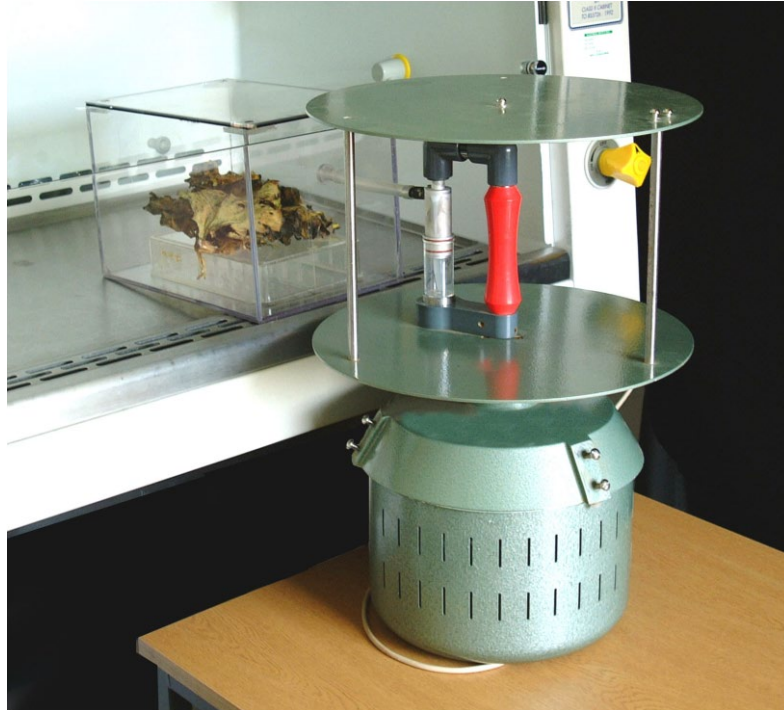
Plate 3. Collection of airborne spora in to an eppindorf vessel using a Burkard cyclone sampler
